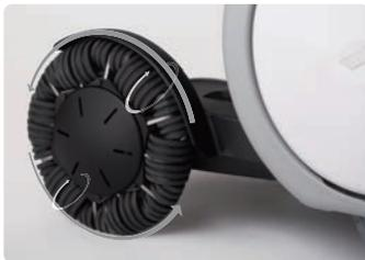
WHILL's patented front Omni-wheels are equally beneficial indoors and out. They allow the Model A to rotate on its axis, maneuver in tight spaces, to cross thresholds and other obstacles and to navigate uneven terrain, all while providing a smooth and comfortable ride. Made up of 24 independent multi-directional rollers Omni-wheels eliminate the need for problematic swiveling casters.
