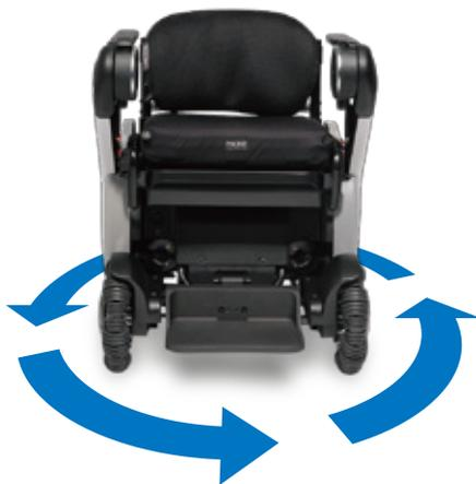
WHILL turns on its own axis with a 28 inch turning radius
